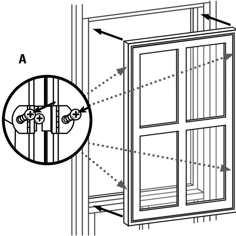
**STEP 1.** Place the fixed utility window sash into the rough opening. Align the pre-drilled holes of the installation clip firmly against the rough opening and fasten the window with 8 pan head aluminum screws (not included) (See Fig A).
