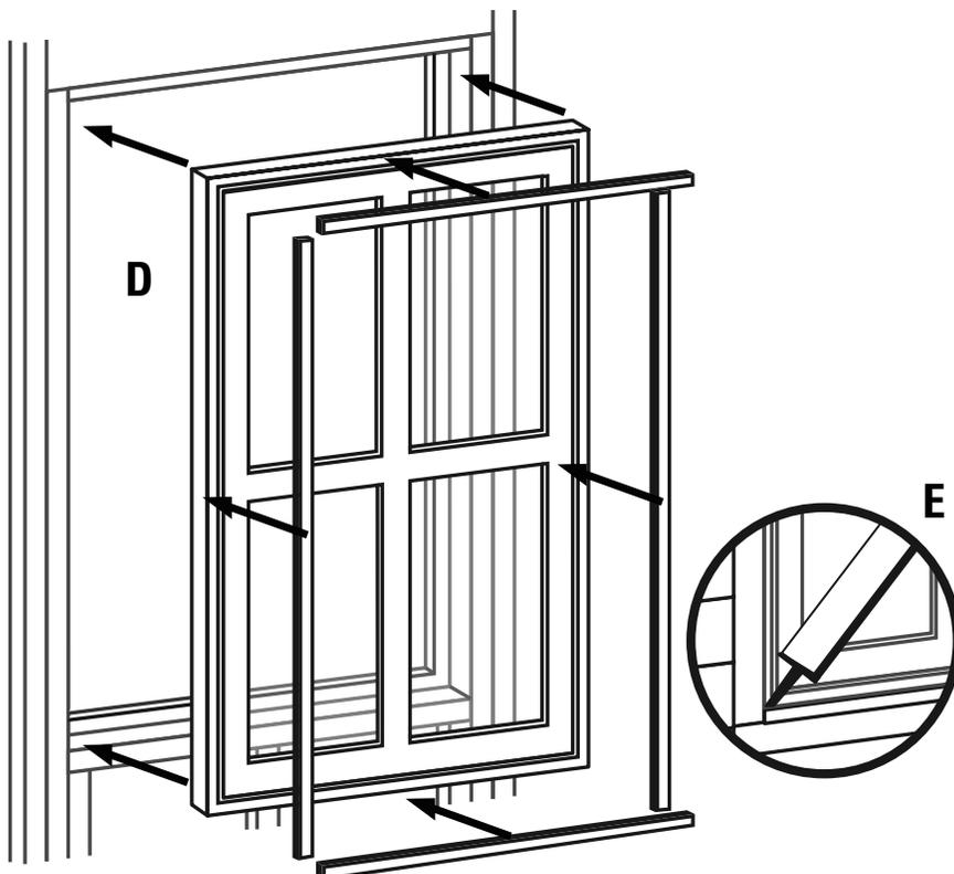
**STEP 2A.** Place the utility fixed window sash in the rough opening. Then install a series of interior stops tightly against the sash wedging the window into place (See fig. D). Finally, seal around the inside and the outside of the window with an approved polyurethane based sealant such as Vulkem® or 100% silicone window and door caulk. Trim the interior and exterior of the window according to your specifications. (See fig. E).
