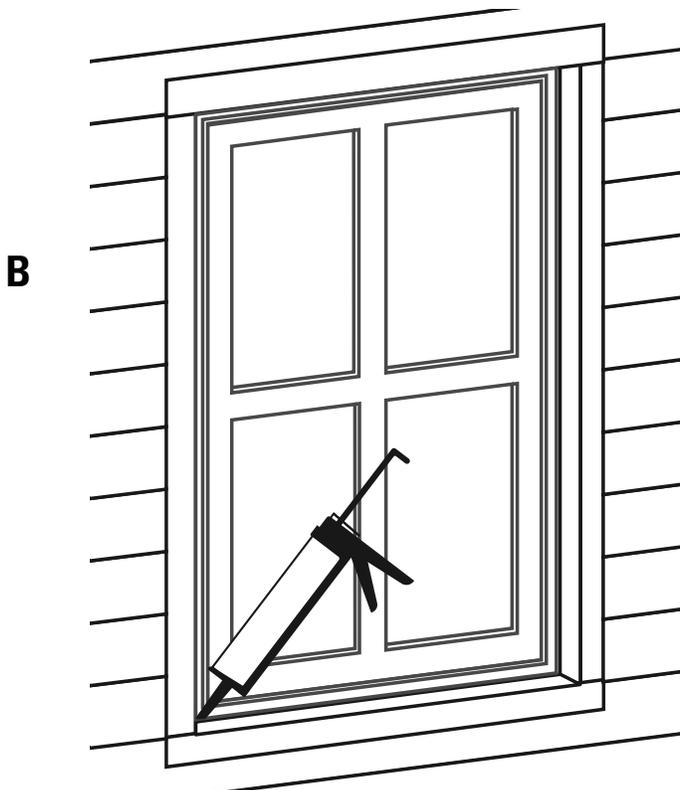
**STEP 2.** Finally, seal around the inside and the outside of the window with an approved polyurethane based sealant such as Vulkem® or 100% silicone window and door caulk. Trim the interior and the exterior of the window according to your specifications (See fig. B).
