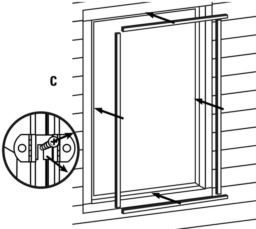
**STEP 1.** If you are not using the pre-installed installation clips simply loosen the set screws, slide the clips out from the side channels and then refasten the set screws. Next, install four 1" x 1/2" stops (strips) towards the outside of the window rough opening frame walls (see fig C).
